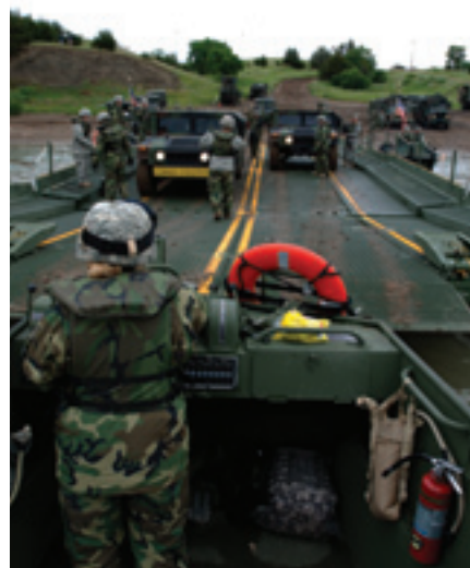
Improved ribbon bridge (IRB)
