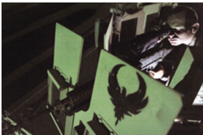
PAS-13 thermal weapons sight mounted on an M-240B machine gun
