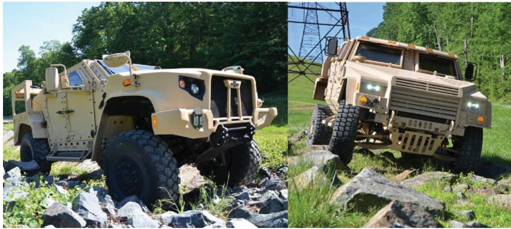
Oshkosh Defense. The JLTV is a tactical wheeled vehicle with a chassis that offers protection from underbelly blasts and a suspension system that can be raised and lowered for off-road conditions. It also boasts greater fuel efficiency than current tactical vehicles. About 100 of the JLTV production vehicles will be provided to the Army and the Marine Corps for testing over the next year.
