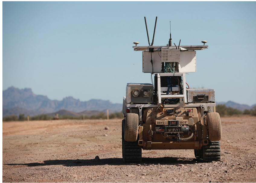
A Robotic Combat Vehicle navigates in the field during Project Convergence at Yuma Proving Ground, Arizona, on 20 October 2021. The Next Generation Combat Vehicle Cross-Functional Team is experimenting with using the vehicle for semi-autonomous resupply, helping Soldiers get the materials they need on the battlefield (U.S. Army photo by Specialist Destiny Jones).
