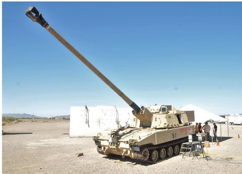
*A prototype M109A7 self-propelled howitzer, modified with the ERCA Armament System, is seen during testing of the five-round Limited-Capacity Autoloader—a technology demonstrator enabling early hardware, software, controls and system integration learning for use in the design and integration of the Full-Capacity Autoloader (U.S. Army photo by Ana Henderson).*
