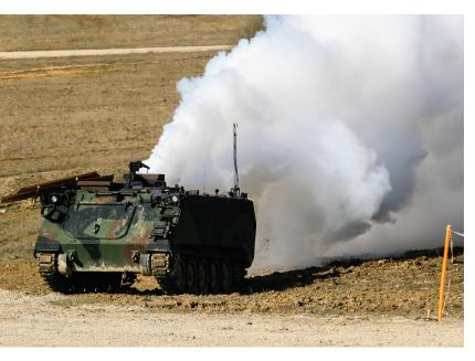
An M58 Wolf is remotely controlled to release a cloud of smoke during a Robotic Complex Breach Concept demonstration at Grafenwoehr Training Area, Germany, 6 April 2018. The Robotic Complex Breach Concept employed the use of RAS in intelligence, suppression, obscuration and reduction missions (U.S. Army photo by Specialist Hubert D. Delany III/22nd Mobile Public Affairs Detachment).
