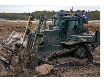
A remote controlled D7R-II dozer removes rubble to create an open lane for vehicles during experimental testing at the Caterpillar Edwards Demonstration and Learning Center in Edwards, Illinois, on 25 October 2018 (U.S. Army Photo by Sergeant 1st Class Jason Proseus/416th TEC).
