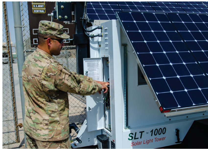
Chief Warrant Officer 3 Cipriano Trujillo, U.S. Army Central Forward Engineering Directorate, sets up the first of 250 solar light towers on 2 October 2015 at Camp Arifjan, Kuwait. The solar lights replaced gas-powered light towers at Camp Arifjan and are part of a larger initiative to conserve energy in the USARCENT area of responsibility (U.S. Army photo by Sergeant James J. Bunn/USARCENT).
