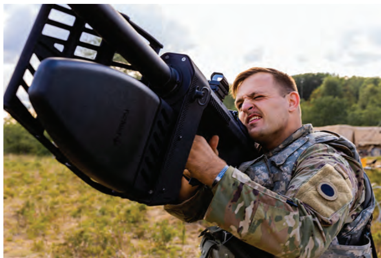
Staff Sergeant Noah Straman, assigned to Headquarters and Headquarters Company, 37th Infantry Brigade Combat Team, fires a DroneDefender during Operation Northern Strike at Camp Grayling, Michigan, 14 August 2022. The DroneDefender incorporates safe, reliable technology that helps defend against unmanned aircraft systems by jamming common frequencies on which they operate (U.S. Army photo by Specialist Benhur Ayetey).
