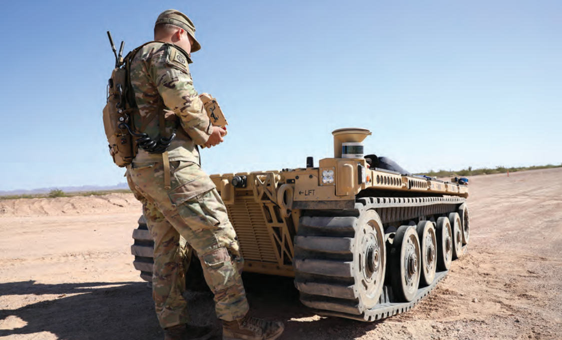
U.S. Army Private First Class Daniel Candales, assigned to the 82nd Airborne Division, uses the tactical robotic controller to control the expeditionary modular autonomous vehicle during a practice exercise in preparation for Project Convergence at Yuma Proving Ground, Arizona, 19 October 2021. During Project Convergence 21, Soldiers are experimenting with using the vehicle for semi-autonomous reconnaissance and resupply (U.S. Army photo by Sergeant Marita Schwab).
