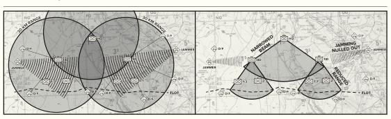
*Figure 11* Comparison of Omnidirectional Antennae with Directional Antennae
