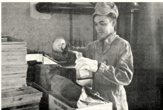
Figure 4. Inspector at volunteer ordnance works takes a sample of Trinitrotoluene (TNT) for testing at an ordnance laboratory (circa 1943). 40
