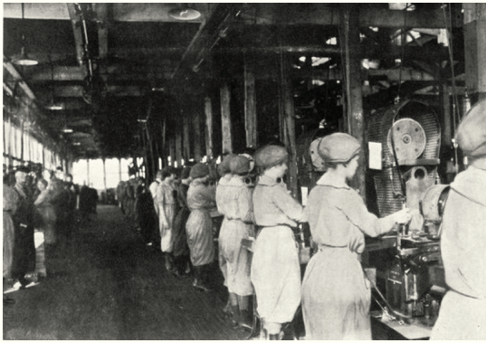
Figure 1. Girls loading point-detonating fuses for high-explosive shells in the body-machining department of a loading plant (circa 1918). 6
