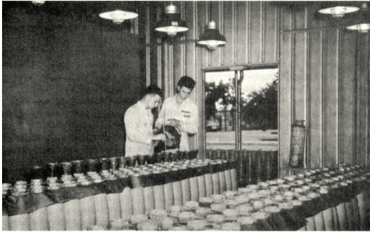
Figure 6. Workmen pouring molten TNT into 155mm shells at the Charleston Ordnance Depot, October 1941. 42
