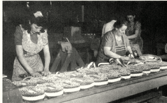
Figure 8. .50-caliber machine gun munitions in fabric belts, being arranged for crating in an ordnance arsenal (circa 1943). 44
