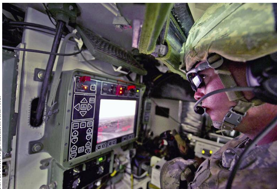
Fire-control system inside an M1126 Stryker infantry carrier vehicle
