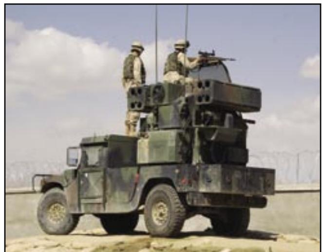
*The Avenger system is a lightweight, highly mobile and transportable surface-to-air missile/gun weapon system. It provides mobile, short-range air defense protection against air and land attacks.*
