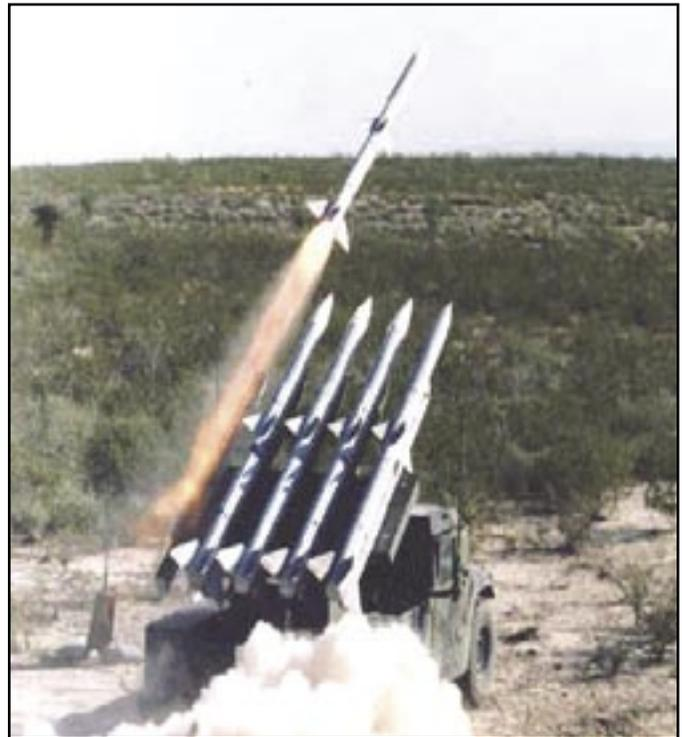
***Surface-Launched Advanced Medium-Range Air-To-Air Missile (SLAMRAAM) provides an extended battlespace, beyond-line-of-sight, non-line-of-sight engagement capability to counter cruise missiles, unmanned aerial vehicles (UAVs), unmanned combat aerial vehicles (UCAVs), and rotary-wing and fixed-wing threat aircraft.***
