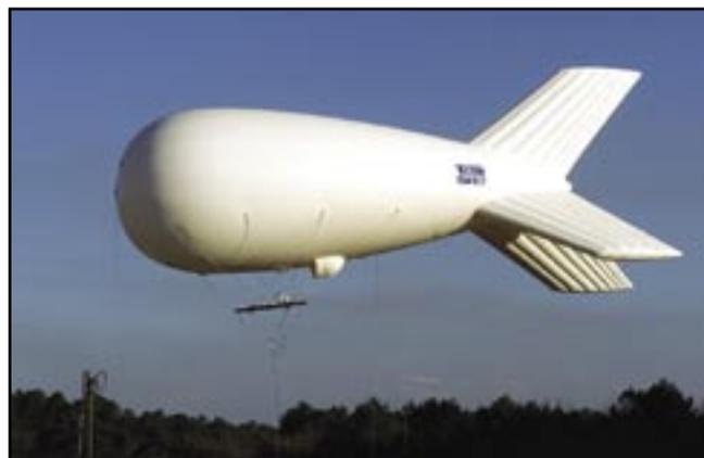
*Joint Land Attack Cruise Missile Defense Elevated Netted Sensor System (JLENS) enhances detection and engagement ranges with air defense weapons such as Patriot, Navy SM-2 missile, Advanced Medium-Range Air-to-Air Missile (AMRAAM) and Medium Extended Air Defense System (MEADS).*
