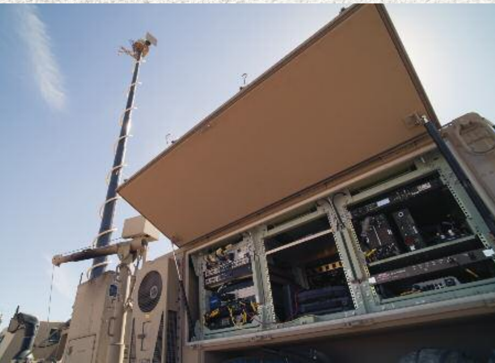
Above, the self-contained Tactical Communications Node (TCN) is the switchboard that provides tactical network communications at a battalion tactical operations center (TOC). Right, soldiers from 1/35 Armor train on dismounted movement to contact battle drills while wearing protective gear for the simulated munitions ammunition being used.
