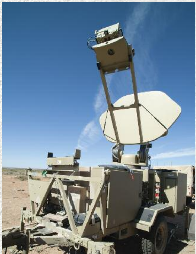
The Satellite Transmission Terminal (Plus) dish provides data transfer for the TCN system.
