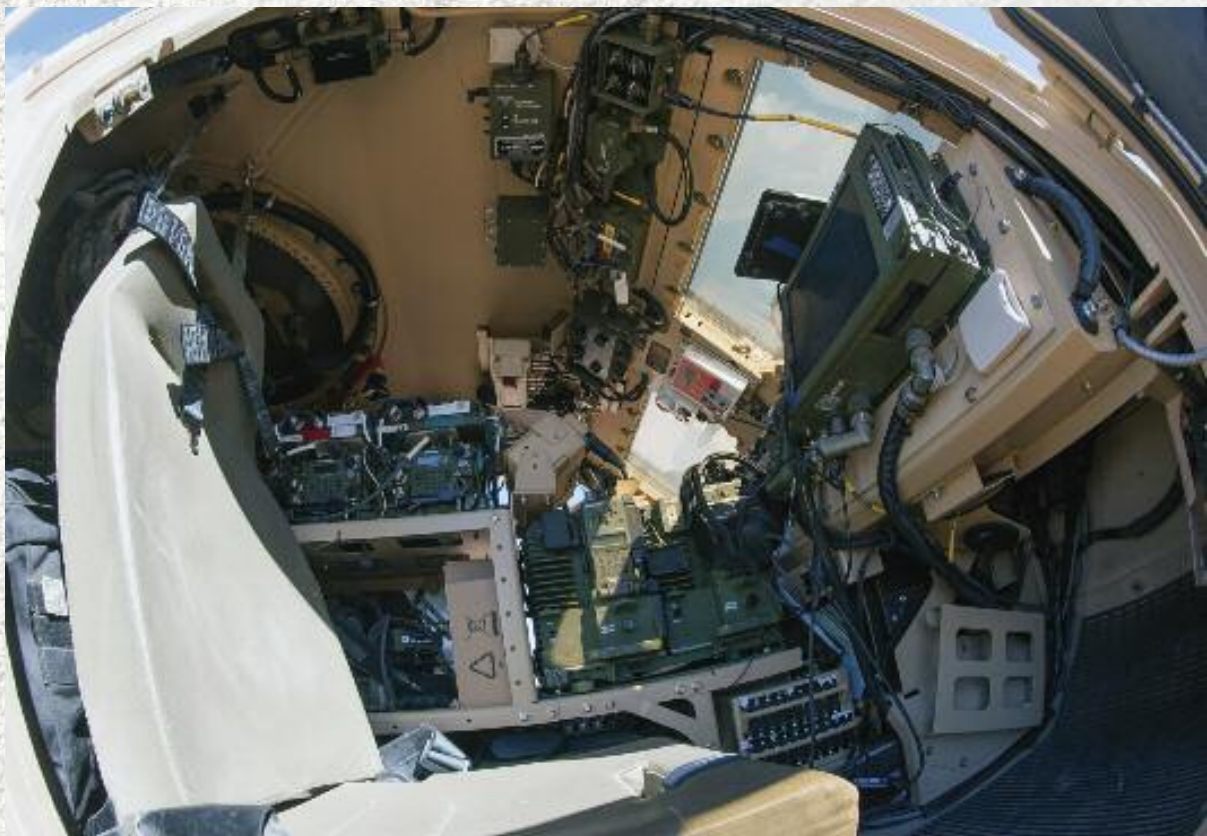
The commander's position in a MATV is crammed with equipment that allows full WIN-T communications capability, giving the commander the same Mission Command information picture that would be available in a TOC. The primary component is the Joint Battle Command Platform.
