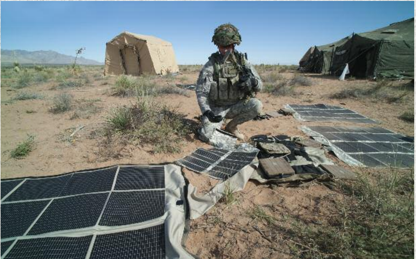
Above, SSG Michael Constantine from the 1st Battalion, 35th Armor (1/35 Armor) charges his Nett Warrior Handheld End User Device with a solar panel kit. The handheld device is the dismantled soldier's component of the Warfighter Information Network-Tactical (WIN-T) system, the primary system being evaluated by the NIE. Right, the smartphone-based device gives soldiers an array of information and communications capabilities in a small package.
