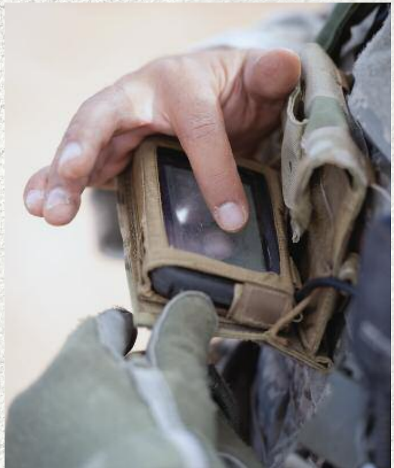
Above, SSG Michael Constantine from the 1st Battalion, 35th Armor (1/35 Armor) charges his Nett Warrior Handheld End User Device with a solar panel kit. The handheld device is the dismantled soldier's component of the Warfighter Information Network-Tactical (WIN-T) system, the primary system being evaluated by the NIE. Right, the smartphone-based device gives soldiers an array of information and communications capabilities in a small package.
