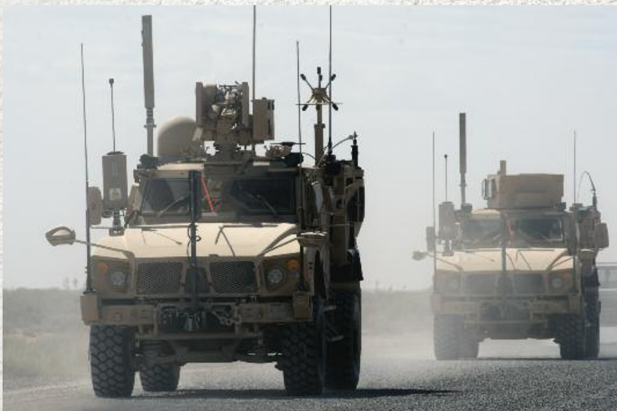
MATVs—mine resistant ambush protected all-terrain vehicles—from the 2nd BCT, 1st Armored Division, relocate to a new position at White Sands Missile Range. The lead MATV is an NIE command vehicle variant.
