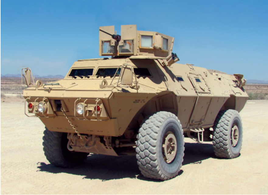
The Mobile Strike Force Vehicle (MSFV) with Gunner's Protective Kit is a modified and updated version of a Textron Machine & Land Systems vehicle platform design, and allows for additional protection while still utilizing commercial off-the-shelf parts.
