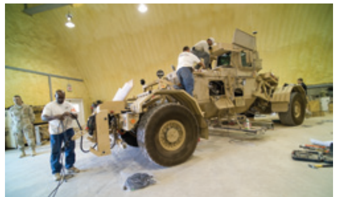
Above, workers upgrade equipment on a Husky metal detecting and marking vehicle at the 401st Army Field Support Brigade (AFSB), Army Materiel Command, maintenance facility at Kandahar. Below, one of the first MRAP all-terrain vehicles to arrive in Afghanistan awaits distribution at the 401st AFSB facility.
