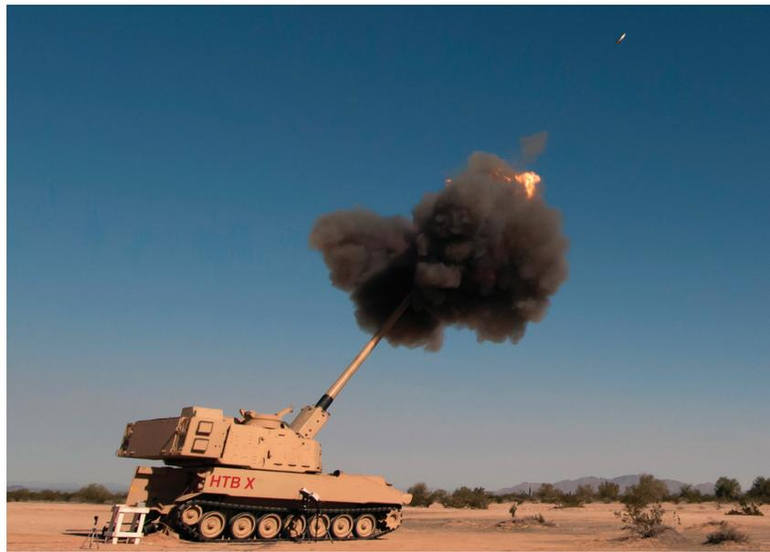
*U.S. Army Yuma Proving Ground (YPG) conducts developmental testing of multiple facets of the Extended-Range Cannon Artillery project, from artillery shells to the longer cannon tube and larger firing chamber that the improved howitzer will need to accommodate them. YPG’s ammunition plant has been instrumental in building multiple experimental formulations, shapes, and configurations for new propelling charges to accommodate the improved projectiles.*
