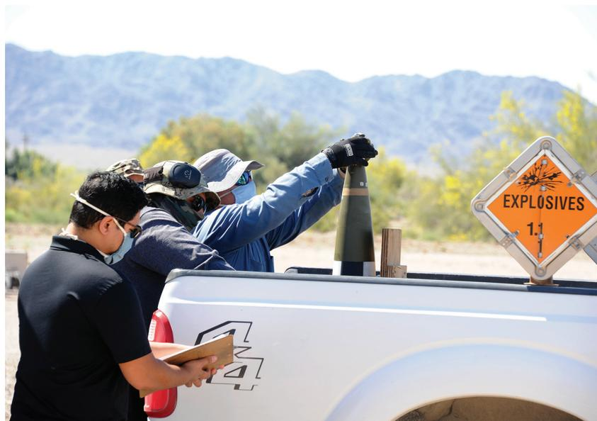
The XM1113 projectile, seen here during testing at Yuma Proving Ground, Arizona, is capable of substantially longer ranges than the currently-fielded 155 mm rounds, thanks to its larger rocket (U.S. Army photo by Mark Schauer).
