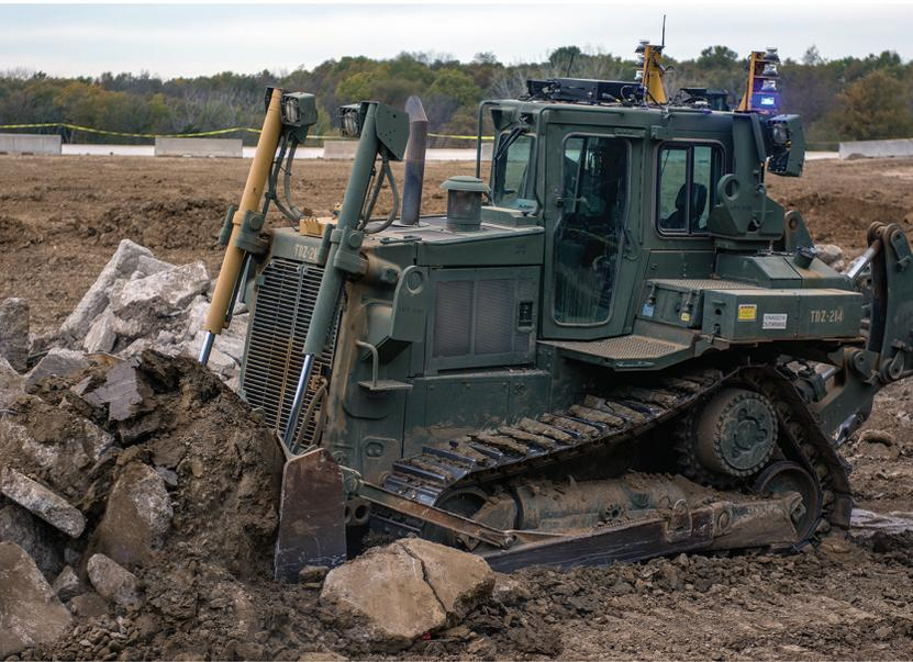
A remote controlled D7R-II dozer removes rubble to create an open lane for vehicles during experimental testing at the Caterpillar Edwards Demonstration and Learning Center in Edwards, Illinois, on 25 October 2018 (U.S. Army Photo by Sergeant 1st Class Jason Proseus/416th TEC).
