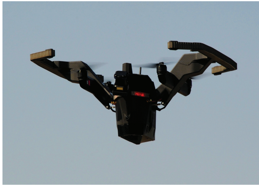
One of the Pegasus family of tactical autonomous systems during testing at Yuma Proving Ground as part of Project Convergence 2020. Pegasus systems have the ability to be used as either unmanned aerial systems (UASs), ground-roving tracked vehicles, or both, as surveillance tools or to create richly detailed 3D maps of an area.
