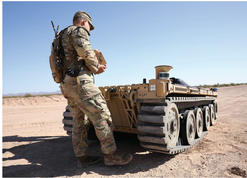
U.S. Army Private First Class Daniel Candales, assigned to the 82nd Airborne Division, uses the tactical robotic controller to control the expeditionary modular autonomous vehicle in preparation for Project Convergence at Yuma Proving Ground, Arizona, 19 October 2021. During Project Convergence 2021, Soldiers experimented with using the vehicle for semi-autonomous reconnaissance and re-supply (U.S. Army photo by Sergeant Marita Schwab).
