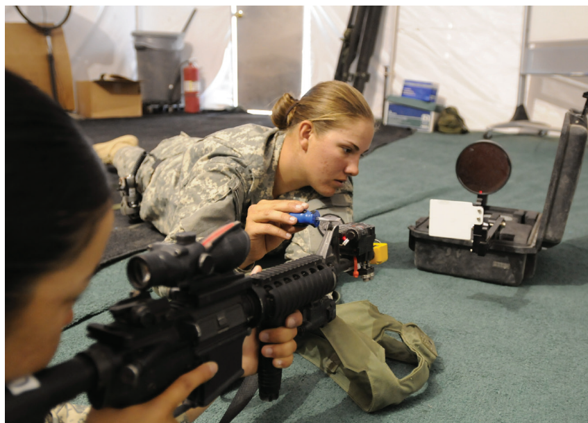
Private First Class Andrea Witmer, Headquarters and Headquarters Troop, 3rd Armored Cavalry Regiment, assists a Soldier with "zeroing" the Multiple Integrated Laser Engagement System attachment on the M-4 rifle. The STE cross-functional team is working to develop modern upgrades to this and other decades-old training systems (U.S. Army photo by Specialist Jennifer Spradlin).
