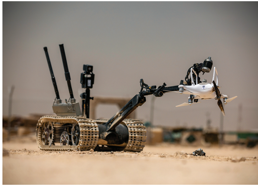
A TALON tracked military robot picks up a downed unmanned aerial system at Al Asad Air Base, Iraq, 19 May 2020 (U.S. Army photo by Specialist Derek Mustard).
