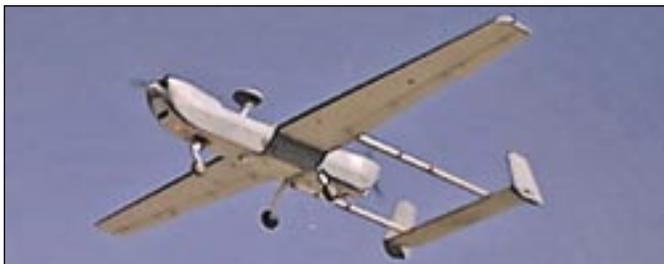
with an Electro-Optic/Infra-Red (EO/IR) sensor or eight hours with a 250-pound payload. The EO/IR—the main payload for the Hunter—is available in both 280mm and 770mm focal lengths. Hunter is the only Department of Defense (DoD) UAV to use a dual-engine system. The MotoGuzzi gasoline engines are being replaced with three-cylinder commercial JP-8 fuel engines. The Army has three Hunter companies deployed with the XVIII Corps, III Corps and V Corps.
