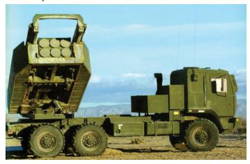
M142 HIMARS. HIMARS is based on the Family of Medium Tactical Vehicles (FMTV) five-ton chassis with a single launch pod. HIMARS is C-130 transportable and rapidly deployable worldwide, fully combat loaded. The system can fire the entire family of MLRS rockets and Army Tactical Missile System (ATACMS) munitions. Currently, seven of 17 battalions have fielded HIMARS.
